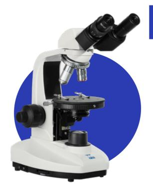
360° revolving stage enables **precise** detection of birefringence
