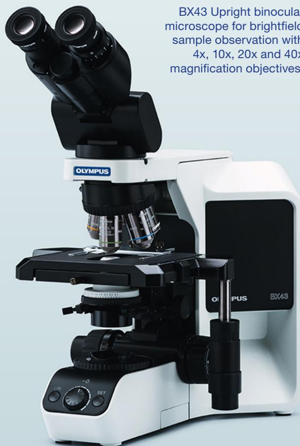
BX43 Upright binocular microscope for brightfield sample observation with 4x, 10x, 20x and 40x magnification objectives.
